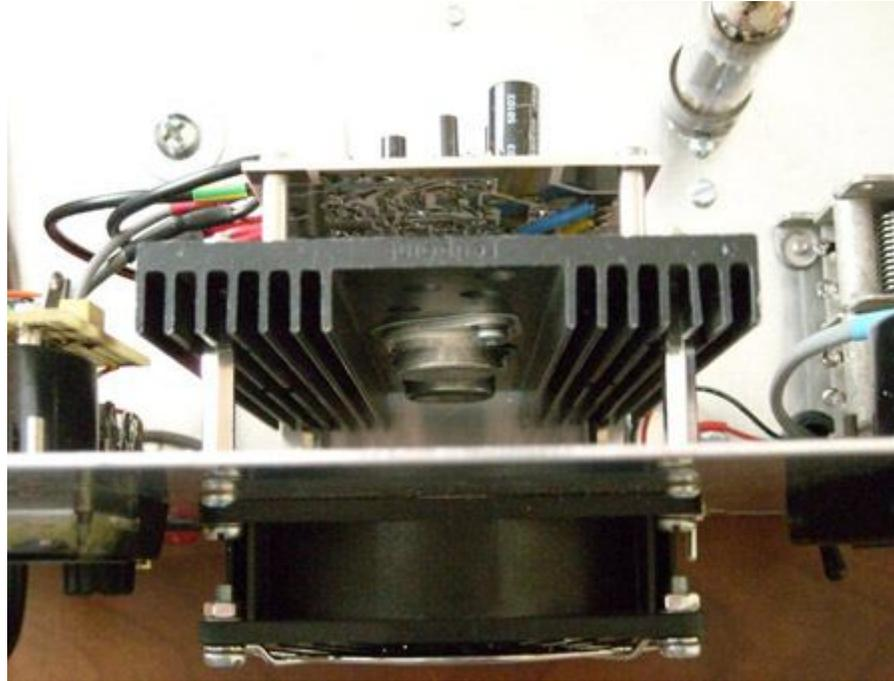
Part of the audio section; the Internal MOSFET (BUZ900/905) 100W RMS into 4 Ohms solid-state Maplin modulator/amplifier. Audio driven by a Band Pass filter; bass cut at 6dB per octave below 200Hz and then flat till 2kHz then rising at 6dB per octave to 5.5kHz then cuts to -40dB by 9 kHz. Of course High Level Anode and Screen Amplitude Modulation with 100% positive and negative peaks available
