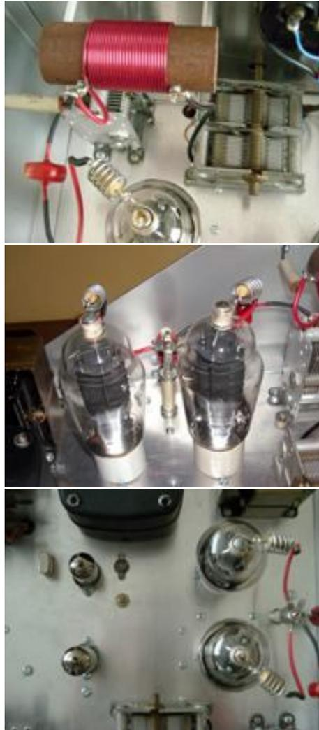
Tank circuit and 2 x 807 Power Amplifier, HT Power Supply is 525 volt / 300 mA
