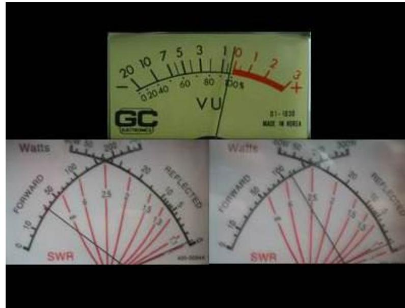
35 Watts minimum if desired... maximum 70 Watt carrier and with Anode and Screen AM PEP will be well over 100 Watts
