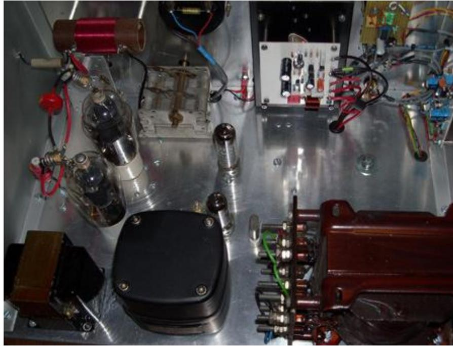
Inside the tube rig; CV5152 Crystal Oscillator, 2 x 807 Power Amplifier, PL84 clamp tube to protect the 807s in case of drive failure. Crystal on the right is the standard HC-6/U type
